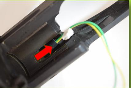
Feed your wire harness through the small hole in the lower receiver as shown in the pictures here. Feed harness in the direction of arrow.
