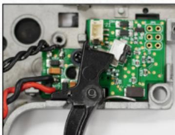
Ensure that the selector plate makes proper contact with the select-fire switch. If the selector plate has a sharp edge, it may be necessary to file it down so it does not damage the select-fire switch. If the selector plate is too wide, it may be necessary to cut a portion so that it can clear the switch when your AEG is set to semi-auto.
