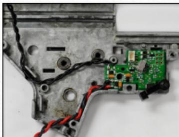
Reattach the trigger and spring, ensuring the trigger makes contact with the trigger switch on the board and the selector plate makes contact with the select-fire switch on the back.
