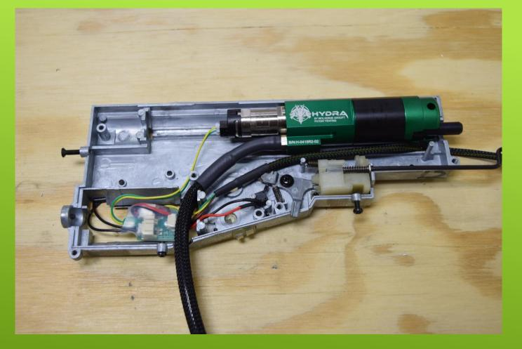
Here is a TM M14 Hydra kit with a Universal Wiring kit installed in the Famas gearbox. Below you will find a closer look at the modifications we have made to the gearbox.
