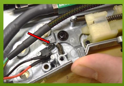
Here you can see the location of the selector switch from the Universal Wiring kit. It's difficult to see in the second picture but we found that we had to add a shim to the selector arm in order to properly engage the microswitch. We ultimately used a piece of eraser and a tad of superglue for this modification. The location of the eraser is indicated by the red arrow.
