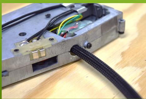
Here we had to drill a hole in the gearbox to make a pathway for the airline. Note that you will need to drill a hole in the body of the gun as well for the line to come out. Be sure to make the holes in the exact same locations or you may have trouble with the line binding or getting pinched between the body and the gearbox.
