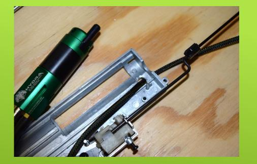
To follow the route of the original electronics in the Famas we drilled a hole in the front of the gearbox to feed the wire harness through. This allows us to put the battery and FCU in the original location of the battery inside the foregrip.
