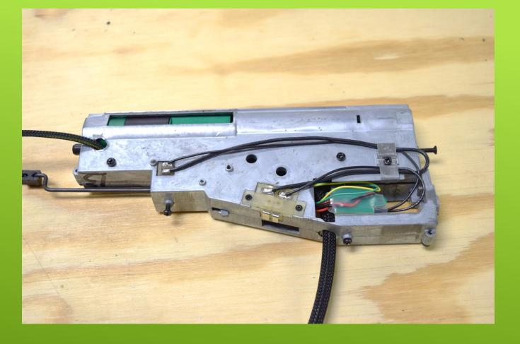
The gearbox is now fully assembled and you can see the modifications we made to it. You can also see where we wired the selector switch and trigger switch into the existing connections.
