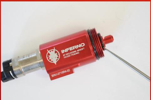
Lubricate\* the 1.5mm x 16mm oring located below the threads and the 1.2mm x 9mm oring located above the threads.
