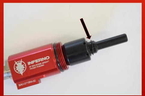
Your Inferno is ready to reassemble. Please remember to install the 1mm x 10mm oring around the nozzle during final assembly.
