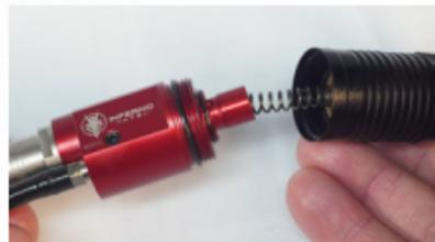
Carefully screw the cylinder clockwise onto the valve housing and hand-tighten it. Pressurize the engine and test for leaks before reinstalling it in your gun.
