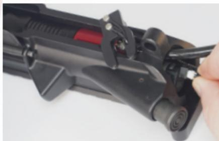
Position the engine so that the retaining groove of the cylinder aligns with the grooves on the upper receiver. The retaining clip and contact yoke should snap into place when correctly aligned.
