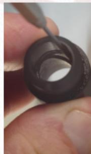
Apply a small amount of lubricant around the circumference of each O-ring.
