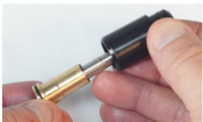
Insert the nozzle and baffle into the valve housing until they are fully seated.
