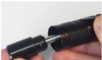
Install one end of the spring into the back of the nozzle and the other into the nose of the valve housing.
