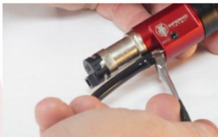
Slide the engine into the upper receiver. Run the contact yoke wire through the receiver and plug it into the solenoid on the rear of the engine.
