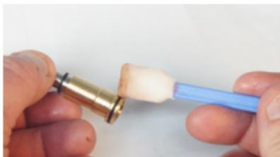
To reassemble, first insert the nozzle into the baffle until it is fully seated.
