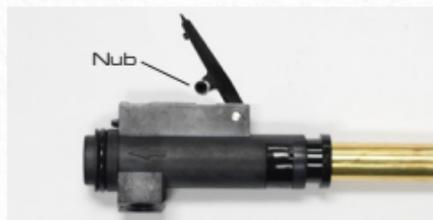
Fit one side of the Hop Adjustment Wheel onto front O-Ring as shown, then press the wheel fully into place. Make sure the hop up arm fits into the channel in the back of the wheel.
