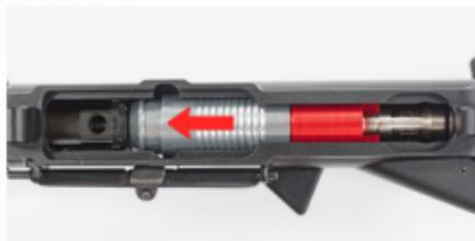
Secure the engine and hop in place with the feed tube assembly.
