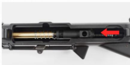
Install the engine so that the nozzle fits into the MTW Hop. Use the engine to push the hop and inner barrel forward into the outer barrel.
