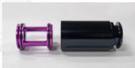
Lubricate all five O-rings on the nozzle cage. There are three 1x19mm O-rings on the outside of the cage and two 1.2x10mm O-rings on the inside.
