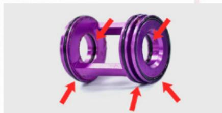
Lubricate the base of the nozzle.
