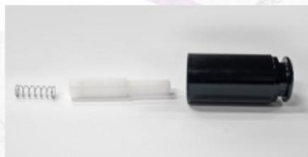
Remove the nozzle cage from the cylinder. You may need to tap the cylinder on your hand or a hard surface to break the cage free from the cylinder.
