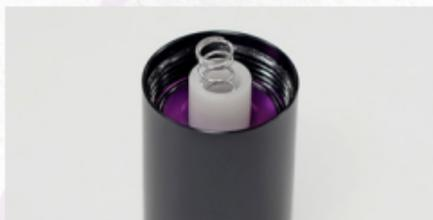
Finally, align the nozzle with valve housing post and push the valve body into the cylinder. Screw the two halves of the unit back together clockwise.
