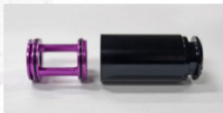
Lubricate all five O-rings on the nozzle cage. There are three 1x19mm O-rings on the outside of the cage and two 1.2x10mm O-rings on the inside.
