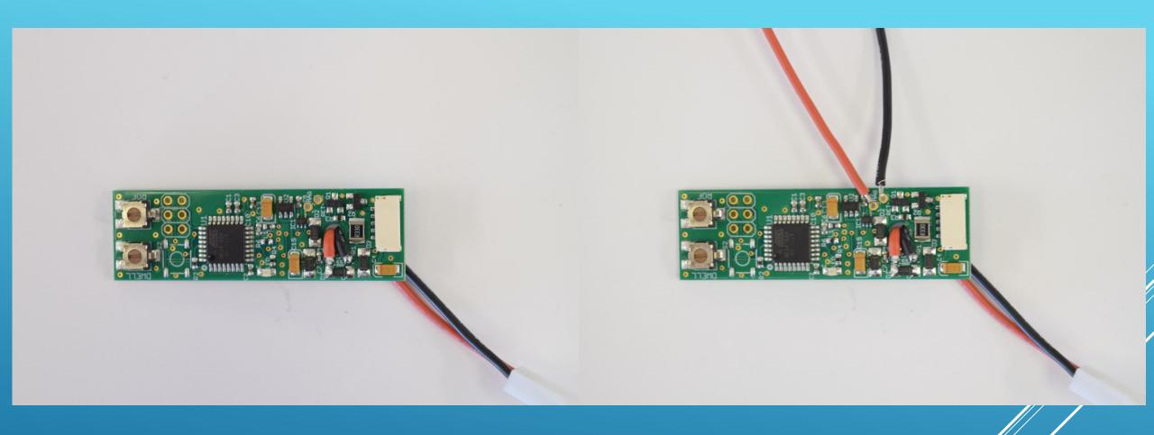
Starting with your standard FCU you will notice there are two connects labled "MAG" (Magazine) and "RET" (Return) respectively. To wire your box mag into the FCU you will solder the red wire into "MAG" and the black wire into "RET".\*
