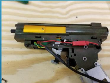
To active full auto with the two stage trigger it was necessary to attach two leads to the connectors on the selector switch as seen in the first photo. These wires were then fed around and through the gearbox and soldered to the pads to complete the circuit. You can see we installed a plug between the two solder points to make disassembly of the gearbox easier.
