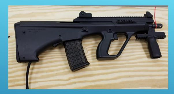
To route the air line, we simply drilled a hole in the lowest point on the stock. We found it easier to install the gearbox if we put an extended air line on the unit; this allows you to feed in the air line before sliding the gearbox into the body.
