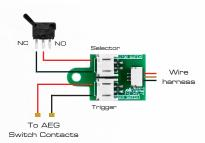
During installation, you may wish to use the clear heat shrink to protect the jumper board and the black shrink tube to protect the wire connections to the microswitch.
