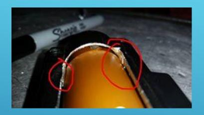
This is not final step however as you will notice that the unit still does not fit squarely inside the gearbox as it should. To finish the modification you will need to file or dremel down the locations marked on the left. This will allow the unit to fit squarely inside the gearbox. Amount to cut down may vary, you will simply need to adjust as you find necessary.
