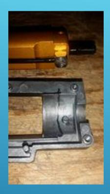
To solve the issue you will need to measure how far back from the front of the gearbox the unit sits and cut away the same length on the plate. You can see an example of where to cut the plate (indicated by a sharpie mark) to the right.
