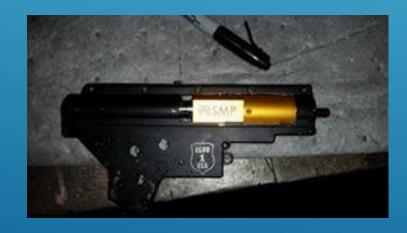
After completion of these modifications your unit should fit squarely in the front of the gearbox. You will also want to re-measure the gearbox to ensure you have the correct nozzle installed in your unit.
