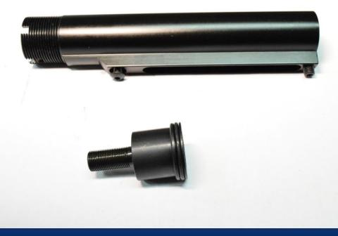
Next you will want to remove the buffer tube adapter. To do this you will just push it through the buffer tube.
