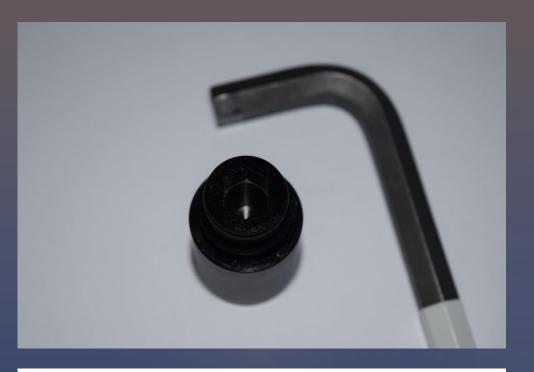
To remove the expansion chamber, use a 3/8 hex key to push the expansion chamber out from the top of the Wraith.
