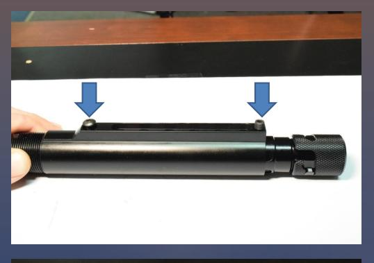
To remove, loosen the 10/32 button head and 10/32 set screw on the bottom of the Wraith buffer tube.
