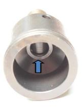
There is also a 1.2mm X 6mm O-ring inside the buffer tube adapter. You will want to make sure to re-lube this Oring as well.
