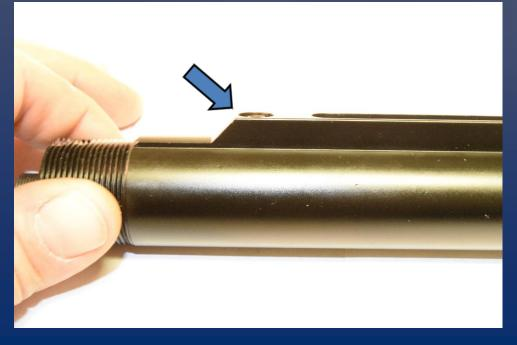
If everything has been aligned correctly you should see the regulator adjustment screw perfectly centered. The 10/32 button head screw should also be recessed.
