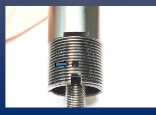
Once you have the buffer tube adapter inserted all the way, you will want to line up the index holes.
