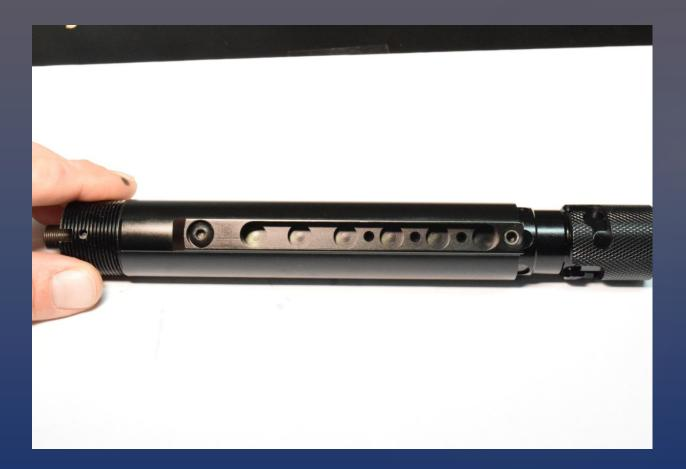
For maintenance on the Wraith Co2 Stock, start by removing the unit from the buffer tube.
