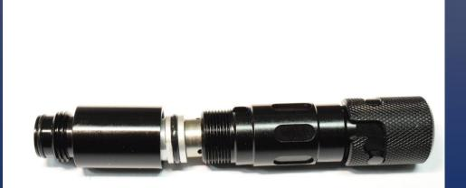
Now you can start by removing the two halves of the Wraith by unscrewing the two parts.
