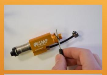
Note: It may not be necessary to replace the orings everytime. If the orings are in good condition skip to slide 7.
