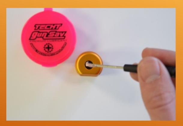
Using a silicon based lubricant\*, apply some to the 1mm x 7mm oring in the cylinder.
