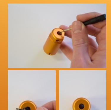
Remove the 1mm x 7mm oring in the cylinder using the microsrewdriver and discard. You will not want to try to reuse this oring as it will likely have Been damaged by the removal process.
