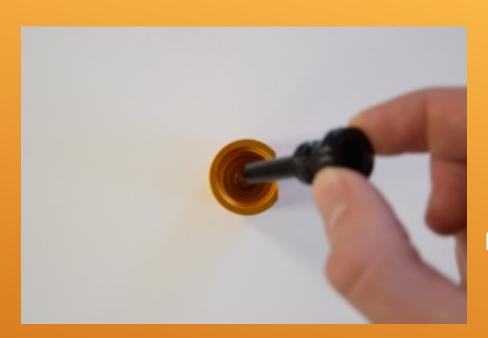
Insert the nozzle into the cylinder and slide it all the way forward.
