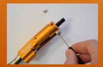
Begin by removing the two set screws located on either side of the SMP with a 1/16<sup>th</sup> in Allen Wrench. Then unscrew the banjo fitting under the nozzle with a flat headed screwdriver.
