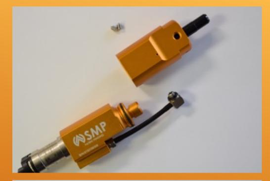
Next, remove the cylinder (front half) of the SMP from The valve body (back half) and remove the nozzle from the cylinder.
