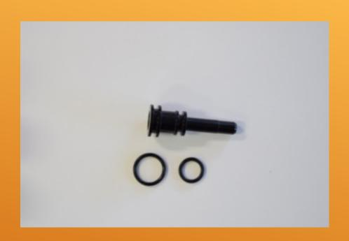
Remove and discard the 2mm x 14mm and 2mm x 10mm orings on the nozzle.
