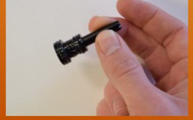
The nozzle and cylinder are now ready to be reassembled.
